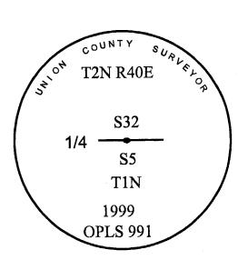
I used a total station with the same basis of bearings as Survey #023-1998 in the establishment of the new accessories. The distances are to the center of the aluminum cap unless otherwise noted.
