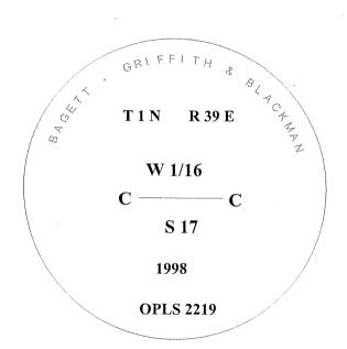
I used a steel tape and magnetic compass in the establishment of the new accessories. I used 16° East declination. Distances are to a 60d spike driven into the root crown of the bearing tree in the right side. A brass washer marked OPLS 83571 was attached to the BT blaze of the new bearing tree.
