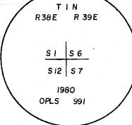
I used a steel tape with a magnetic compass with 20 degree East declination. I set a brass washer marked OPLS 991 at the BT. blaze.
