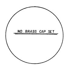
I used a steel tape and a magnetic compass with 200 E declination. I also set brass washers marked OPLS 991 at the BT blaze.
