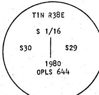
Brass washer nailed to BT Blaze. Used steel tape and magnetic compass with 17° E declination. Distance measured to center of tree.
