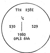
Brass washer nailed to BT blaze. Used steel tape and magnetic compass with 17°E declination. Distance measured to center of tree.
