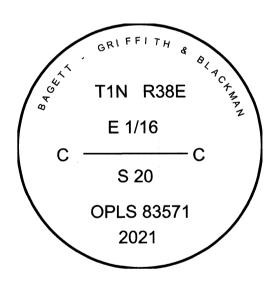
I used a steel tape and magnetic compass in the establishment of the new accessories. I used 14° East declination, the bearings are to a brass washer marked OPLS 83571 in the BT blaze. Distances are to a 60d spike in the right side of the root crown of the Douglas Fir and to an aluminum nail in the right and side of the Larch.
