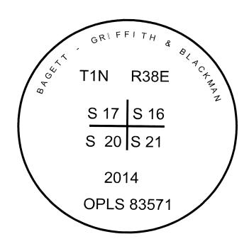
I used a steel tape and magnetic compass in the establishment of the new accessories. I used 16° East declination, the distances are to a 60d spike in the right hand side of the bearing trees. Bearings are to a washer marked OPLS 83571 set in the upper portion of the BT blaze.
