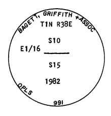
Used steel tape and magnetic compass with 20° declination. Distances measured to center of tree.
