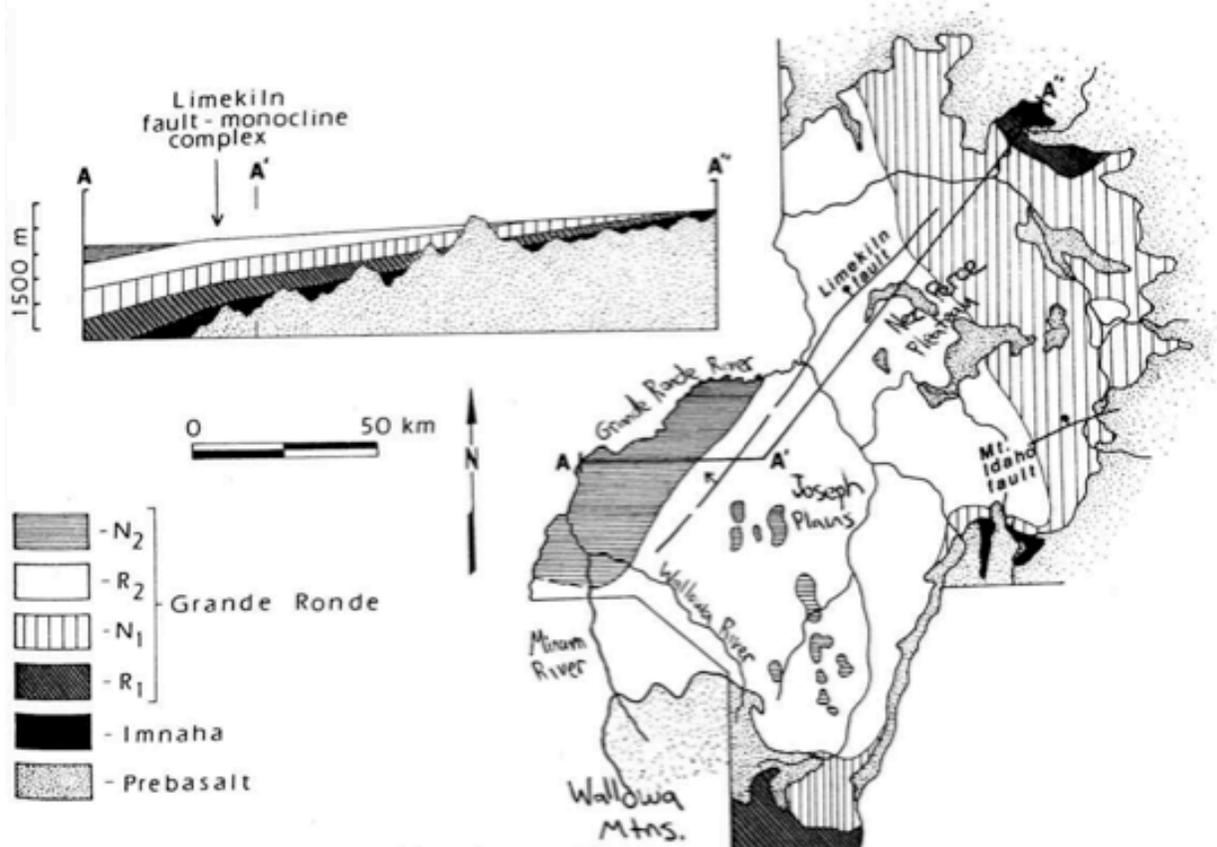
**Figure 7.** Map view and cross-section of the southeast part of the Columbia River Basalt Group immediately after eruption of Grande Ronde Basalt. (modified from Camp & Hooper 1981)
