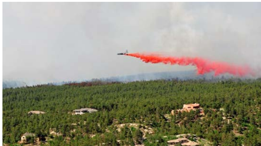
Aircraft applying slurry to try to protect a subdivision built in the wildland-urban interface of Colorado Springs, Colorado, from the approaching 2013 Black Forest Fire. Photo credit: U.S. Army photo by Sgt. Jonathan C. Thibaut
